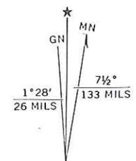
UTM GRID AND 1972 MAGNETIC NORTH DECLINATION AT CENTER OF SHEET
