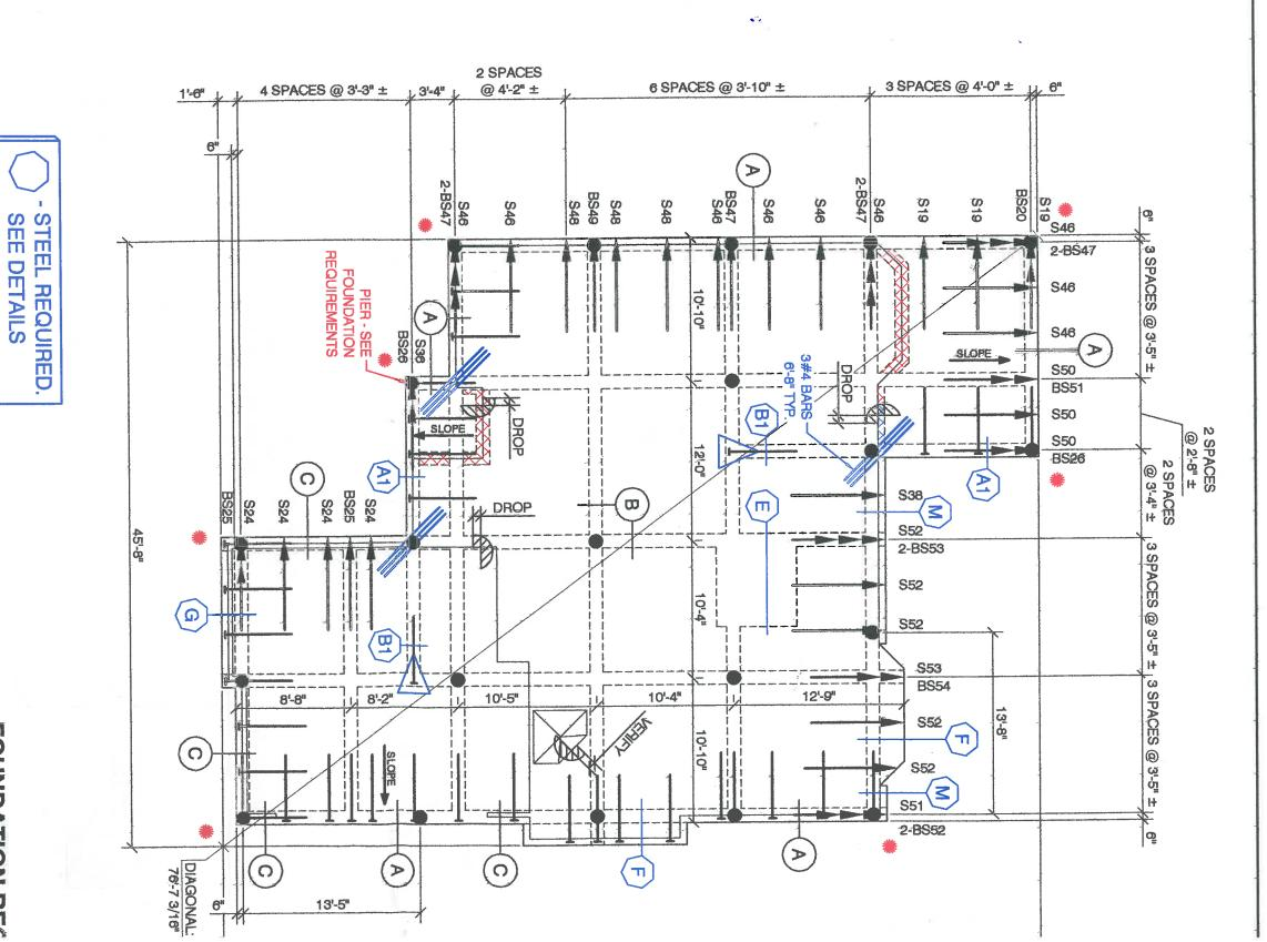
**\*\*** CAUTION: VIBRATE ALL CABLE LIVE AND DEAD ENDS TO ENSURE MAX. DENSITY CONCRETE, ESPECIALLY AREAS WHERE MULTIPLE
