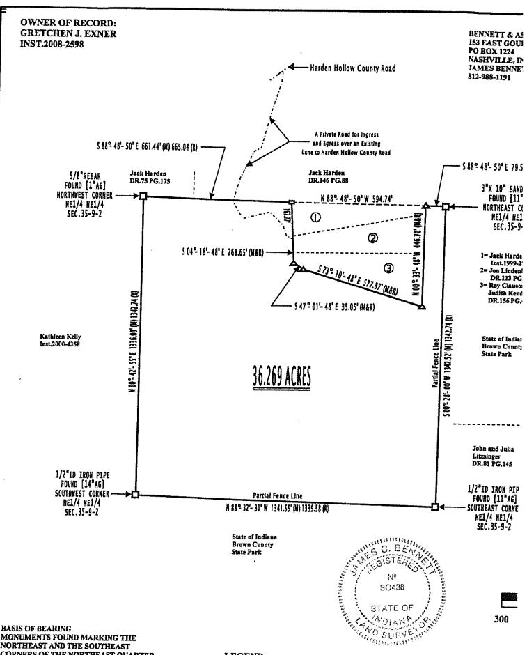
MONUMENTS FOUND MARKING THE NORTHEAST AND THE SOUTHEAST CORNERS OF THE NORTHEAST QUARTER OF THE NORTHEAST QUARTER OF THE NORTHEAST QUARTER OF SECTION 35, TOWNSHIP 9 NORTH, RANGE 2 EAST WERE ROTATED TO SOUTH 00 DEGREES 28 MINUTES 00 SECONDS WEST TO MATCH DEED BEARINGS.
