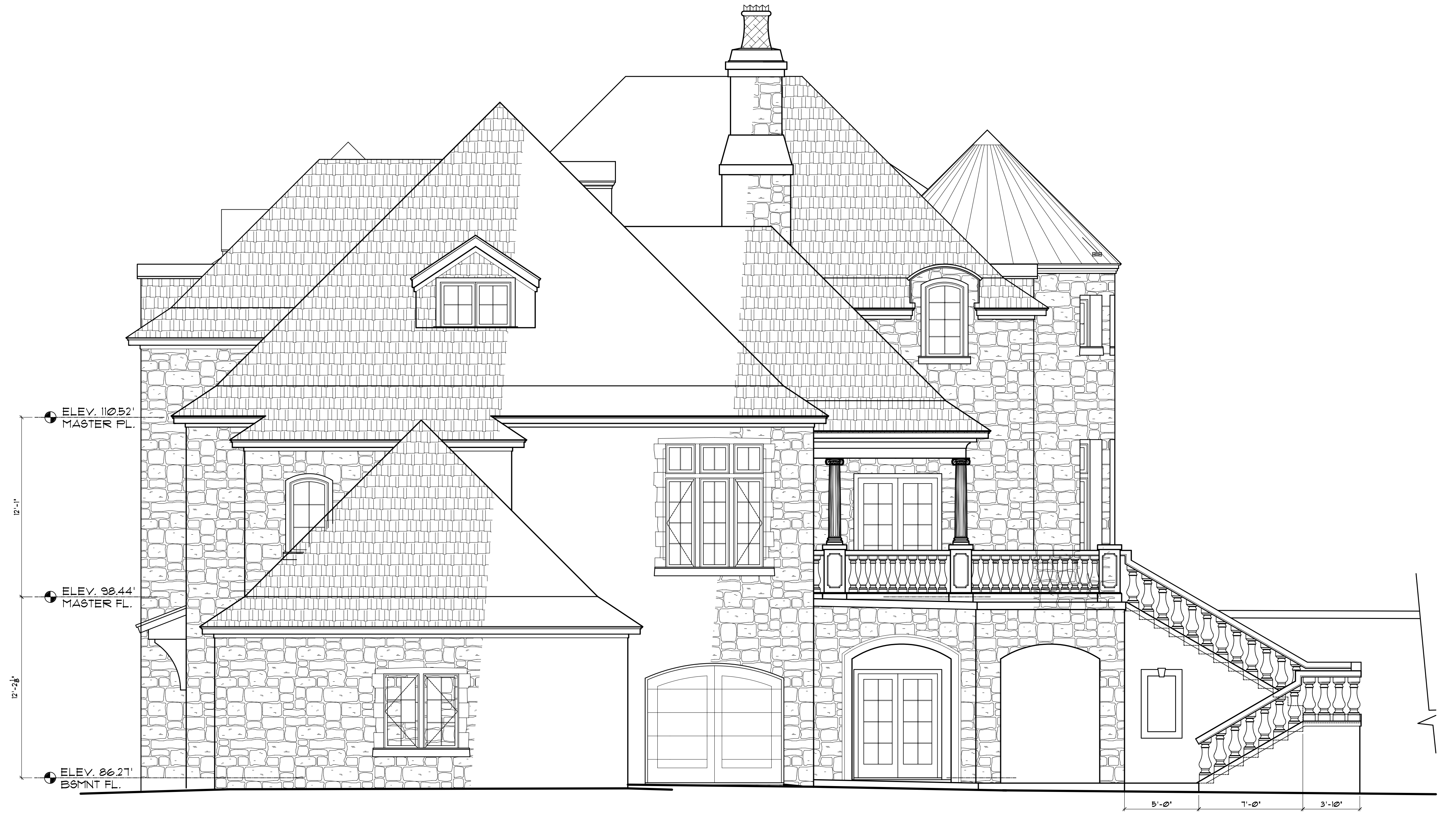
SOUTH ELEVATION AT GARAGE A-B SCALE 1/4"=1'-0"
