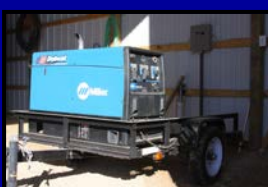
MILLER BOBCAT 250 WELDER/GENERATOR
