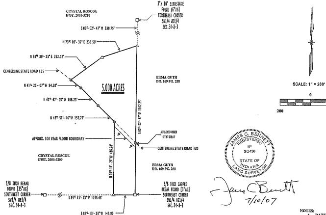
BASIS OF BEARING MONUMENTS FOUND MARKING THE NORTHEAST AND THE SOUTHEAST CORNERS OF THE SOUTHWEST QUARTER OF THE NORTHEAST QUARTER OF SECTION 34 TOWNSHIP 8 NORTH RANGE 3 EAST WERE ROTATED TO SOUTH 00 DEGREES 02 MINUTES 47 SECONDS WEST TO MATCH ADJOINING DEED BEARINGS.
