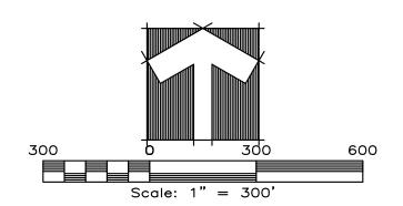
BEARINGS BASED ON TEXAS STATE PLANE COORDINATE SYSTEM, CENTRAL ZONE NAD 83.
