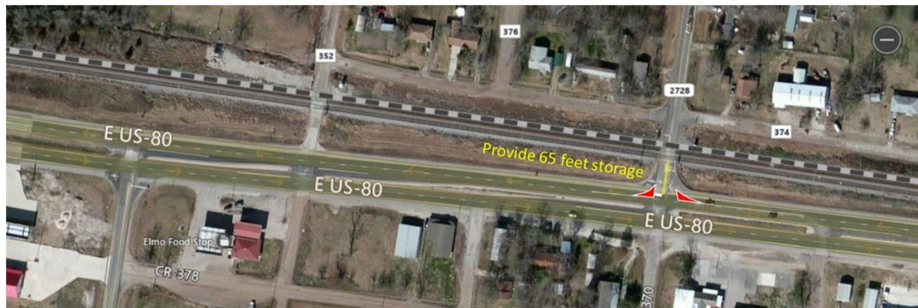
Figure 21. Improvement S3 to Channelize the Intersection of FM 2728 at US 80 Improve Truck Storage and Intersection Operations
