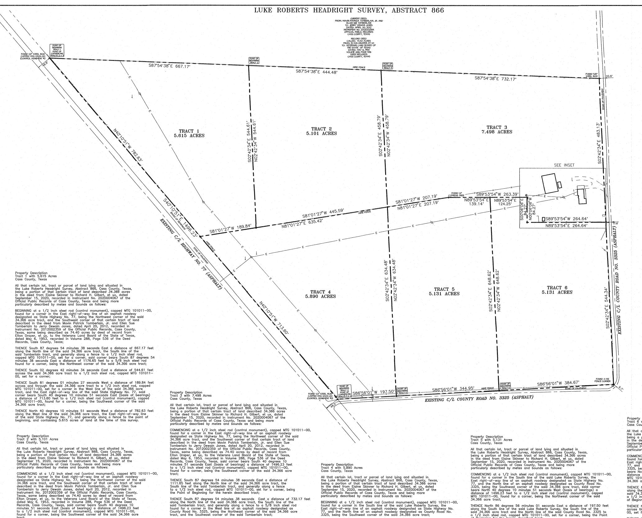
THENCE South 02 degrees 42 minutes 34 seconds East a distance of 483.13 feet along the East line of the said 34.366 acre tract, and the West line of the said County Road No. 3325 to a 1/2 inch steel rod, capped MTG 101011-00, set for a corner, said corner bears South 02 degrees 42 minutes 34 seconds East a distance of 544.34 feet to a cross—tie fence corner post found for a corner,
