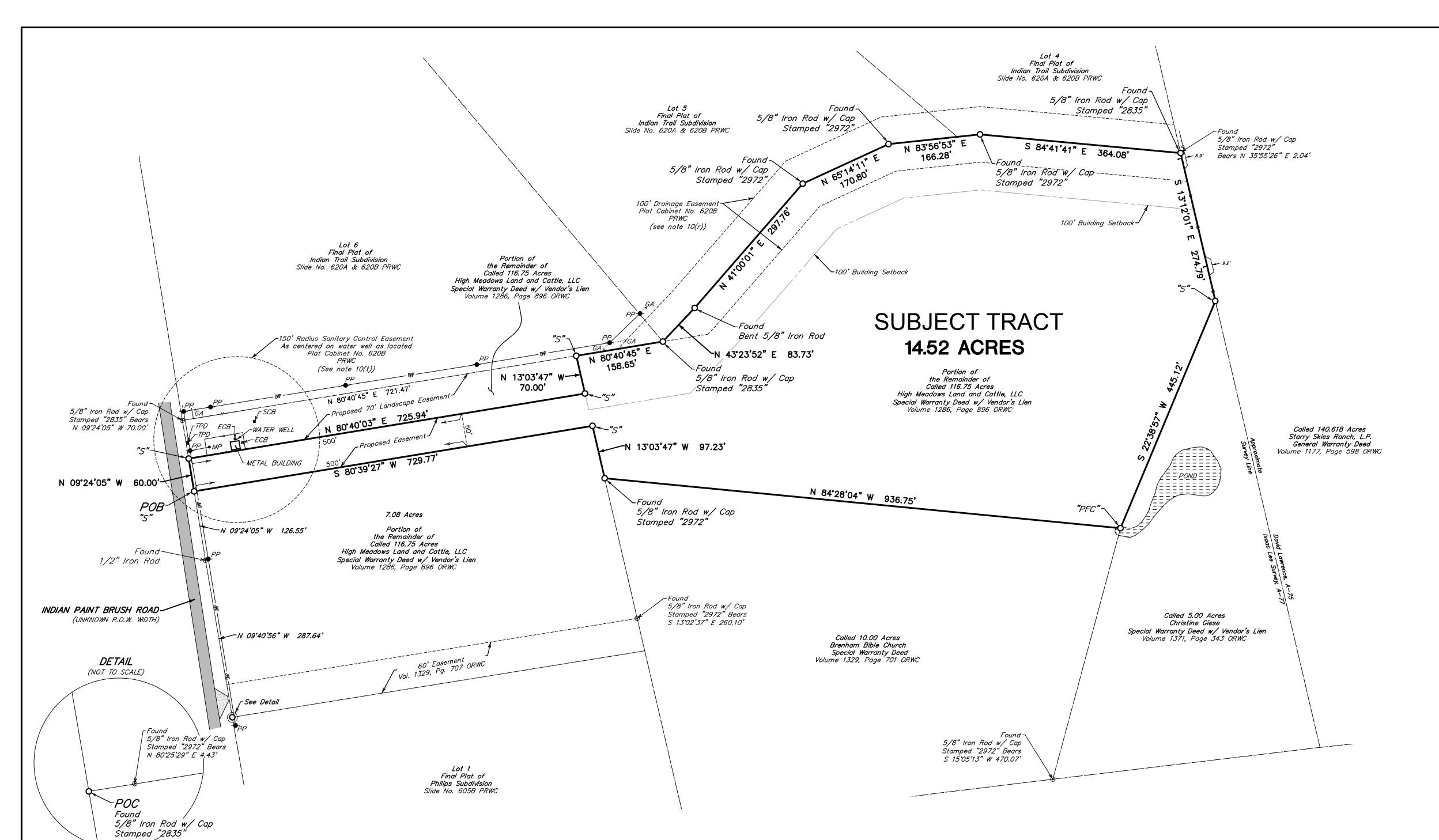
LEGEND: ELECTRIC CONTROL BOX ECB GUY ANCHOR ORWC OFFICIAL RECORDS OF WASHINGTON COUNTY POINT-FOR-CORNER PLAT RECORDS OF WASHINGTON COUNTY POB POINT OF BEGINNING POINT OF COMMENCING POC POWER POLE RIGHT-OF-WAY SET 5/8" IRON ROD (WITH CAP STAMPED "JONES&CARTER") SPRINKLER CONTROL BOX TELEPHONE PEDESTAL VOLUME ASPHAL<sup>®</sup> WATER SCALE: 1" = 100'100 ADJOINER LINE 200 **BOUNDARY LINE** CHAIN LINK FENCE EASEMENT LIMITS HOG WIRE FENCE OVERHEAD POWER WOOD FENCE
