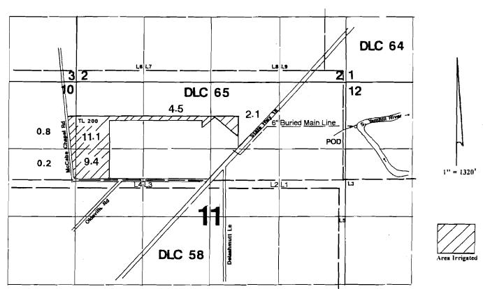
Pt. of Diversion is located 850'S & 180'E from the NW corner of Section 12.
