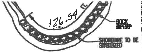
PLAN SHOWING STABILIZED SHORELINE
