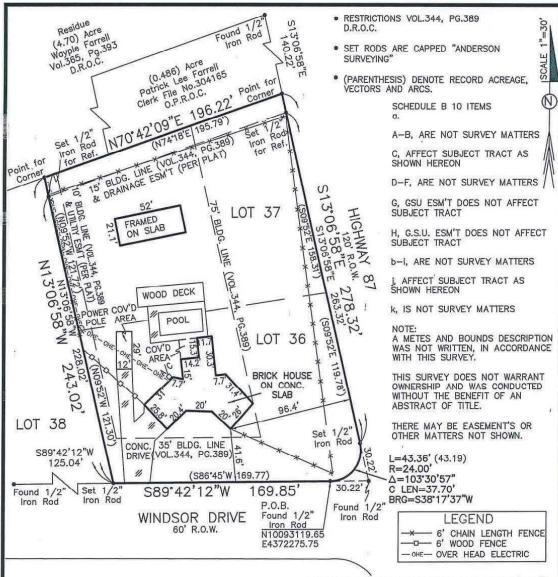
Property location in relation to Flood map was determined by scale, actual field elevation not determined unless noted. Anderson Surveying, does not warrant nor subscribe to the accuracy of said map. Coordinates, Bearings, and Distances are based on the State Plane coordinate grid system, Texas Central Zone 4203, NAD83, having a convergence angle of 0.3 Deg. 23 Min. 08 Sec., and may be converted to surface by multiplying by a combined scale factor of 0.999985435.
