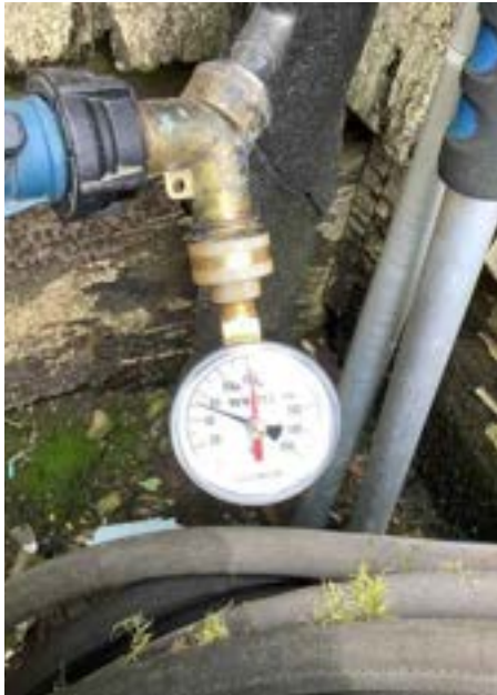
Water Pressure Readings Observed Between 55 & 60 PSI
