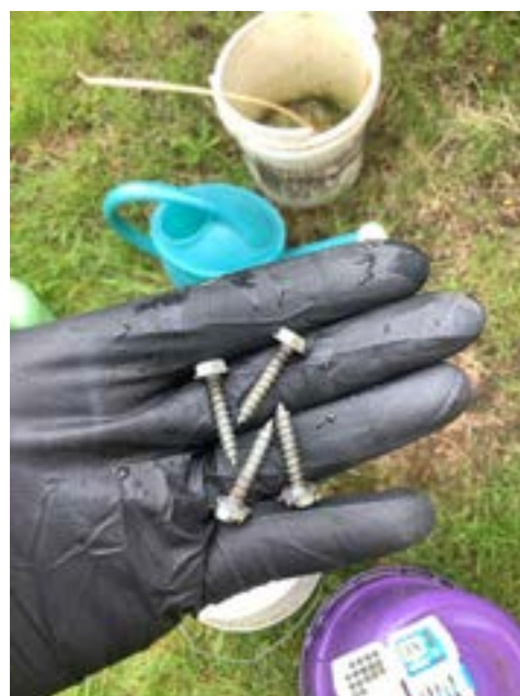
Incorrect Type of Panel Cover Fasteners - Side B
