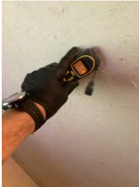
Ceiling Surface Staining/Discoloration - Full Bathroom (First Floor)
