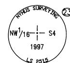
NORTHWEST 1/16 CORNER SECTION 4 SET: A PIPE WITH BRASS CAP, MARKED AS SHOWN, 0.3' ABOVE GRADE, FROM WHICH; A 5" FIR. SCRIBED "NW1/16 S4 BT" ON A DOUBLE BLAZE, BEARS N17'W, 12.1' A 12" SPRUCE, SCRIBED NW1/16 S4 BT" ON A DOUBLE BLAZE, BEARS S87°É, 18.1'
