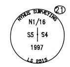
NORTH 1/16 CORNER TO SECTIONS 4 & 5 SET: A PIPE WITH BRASS CAP, MARKED AS SHOWN, 0.5' ABOVE GRADE, FROM WHICH; A 16" SPRUCE, SCRIBED "N1/16 S5 BT" ON A DOUBLE BLAZE, BEARS \$39'W, 28.9' A 70" SPRUCE, SCRIBED "N1/16 S4 BT" ON A DOUBLE BLAZE, BEARS N69'E, 77.1
