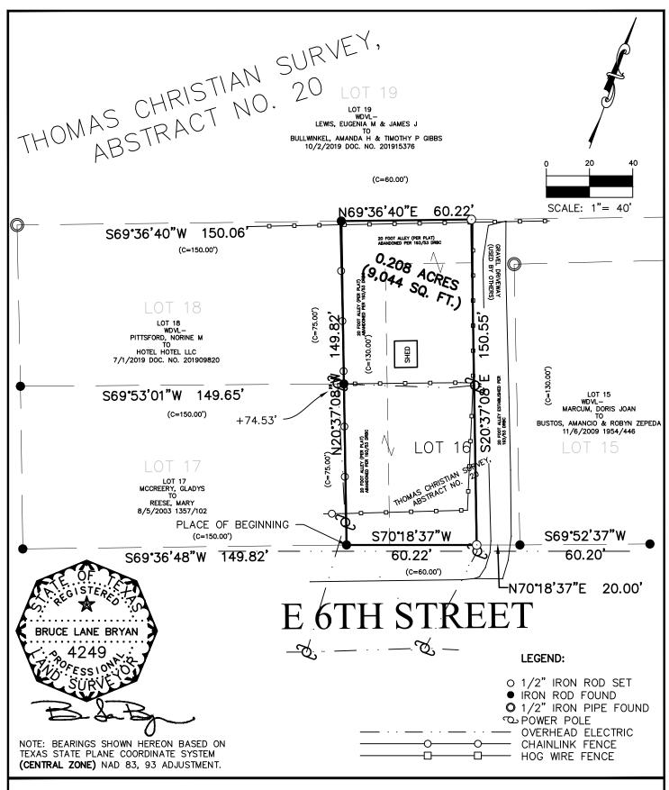
THIS IS TO CERTIFY THAT, ON THIS DATE, A TRUE AND ACCURATE SURVEY WAS MADE ON THE GROUND UNDER MY SUPERVISION OF PROPERTY LOCATED AT **E. 6TH STREET** IN BASTROP COUNTY, TEXAS, DESCRIBED AS FOLLOWS: **LOT SIXTEEN (16) OF NORTH TERRACE**, AN ADDITION IN BASTROP COUNTY, TEXAS, ACCORDING TO THE MAP OR PLAT RECORDED IN CABINET 1, PAGE 3A, OF THE PLAT RECORDS OF BASTROP COUNTY, TEXAS.
