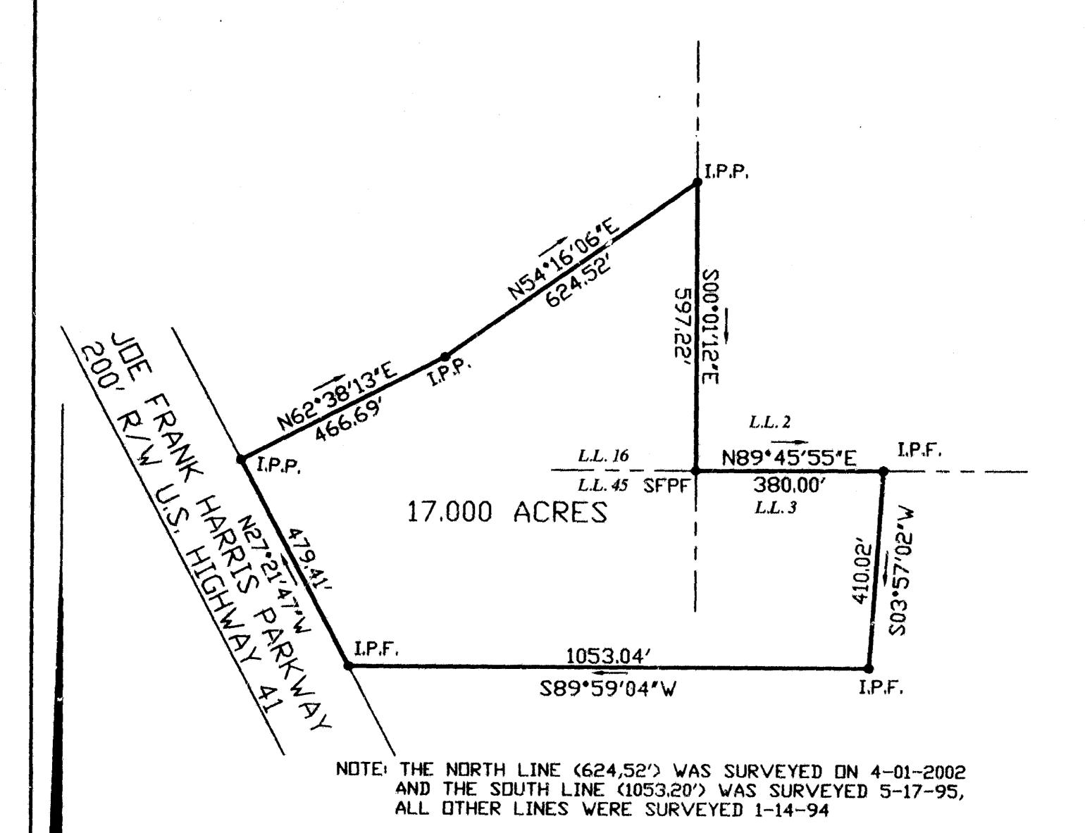
FIELD TRAVERSE: CLOSURE; ONE FOOT IN 10,000 FEET USING A LIETZ SET 3. ANGULAR ERROR; 0'00'06" PER ANGLE POINT USING A LIETZ SET 3. ADJUSTED; USING THE COMPASS RULE.
