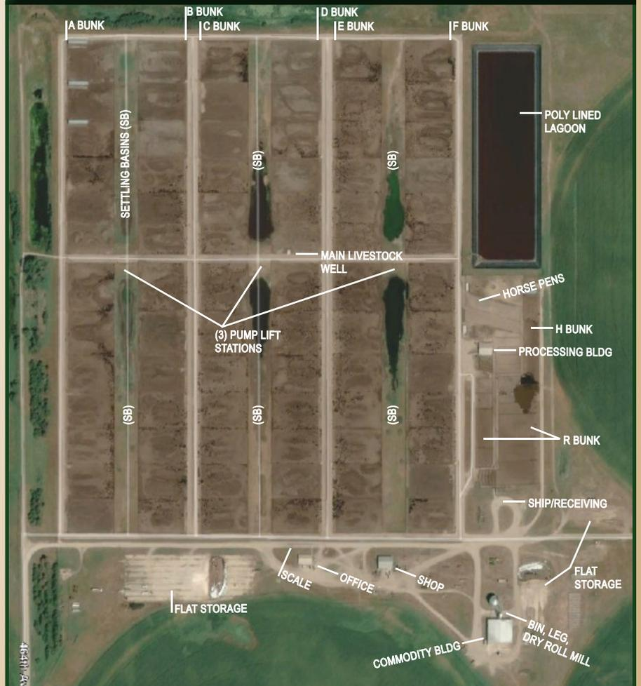
Dewatering of the lagoon is accomplished via a pumping station that delivers water via underground pipe to the southeast pivot quarter of the subject and a neighboring pivot quarter directly to the north of the feedyard facility.
