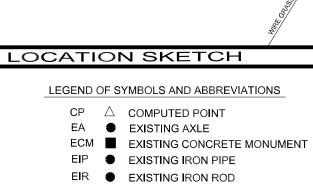
NIR O NEW IRON ROD FIRE HYDRANT GAS VALVE POWER POLE LIGHT POLE SANITARY SEWER MANHOLE STORM MANHOLE TELEPHONE PEDESTAL TRANSFORMER WATER METER WATER VALVE **W** ABOVE GRADE BG CB CL CO **BELOW GRADE** CATCH BASIN CENTERLINE CLEAN OUT CORRUGATED METAL PIPE CORRUGATED PLASTIC PIPE DROP INLET CPP
