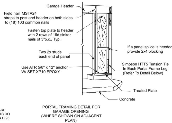
PORTAL FRAMING DETAIL FOR GARAGE OPENING (WHERE SHOWN ON ADJACENT PLAN)
