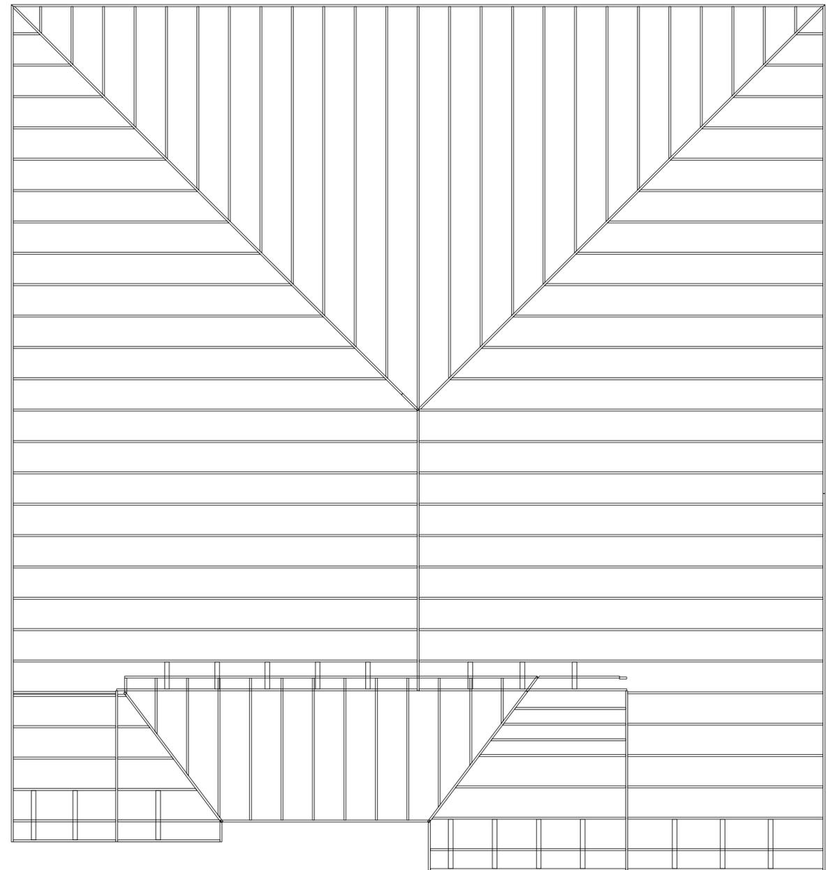
**Roof Layout & Framing Plan**
