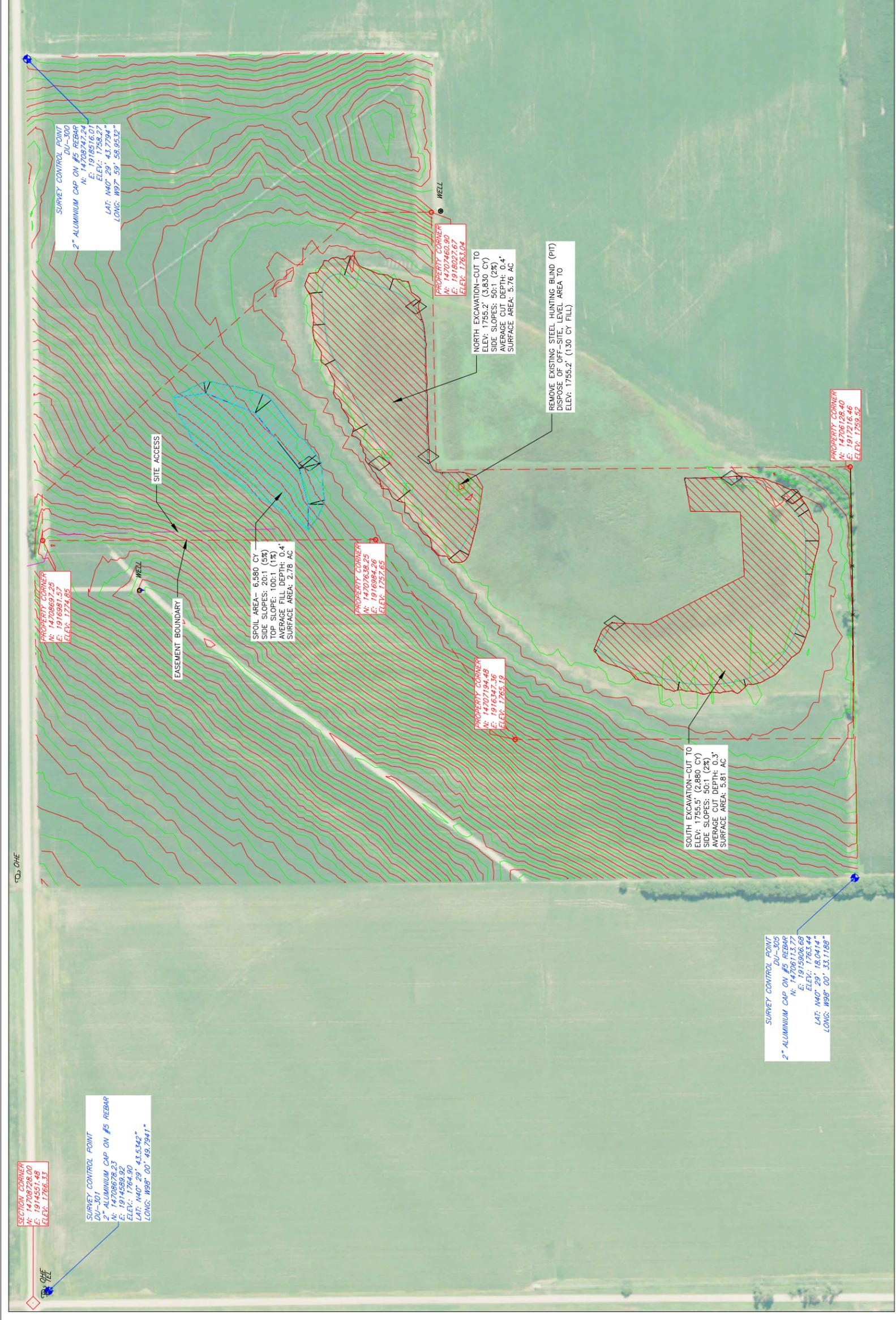
SEEDING AND MULCHING NOTE: THE CONTRACTOR IS RESPONSIBLE FOR PROVIDING AN ADEQUATE SEED BED TO ALLOW SEEDING WITH STANDARD SEEDING EQUIPMENT. THIS WILL INCLUDE USE OF A HARROW OR OTHER MEANS IN ORDER TO LEAVE A SMOOTH, TRACK-FREE FINISH. BACK DRAGGING WITH A DOZER IS NOT AN ACCEPTABLE FINISH.
