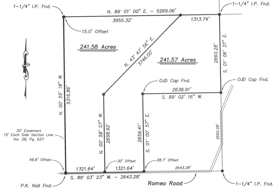
Bearings based on U.S. State Plane of 1983 "Texas North Zone" -#4201 Distances are Ground Distances Grid to Ground Scale Factor = 1.00021
