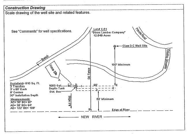
Show the property lines, all existing and proposed structures, existing and proposed sewage systems and water supplies, slope, and any topographic features which may impact the design of the well.
