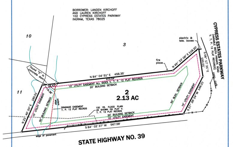
THIS PLAT REPRESENTS A SURVEY MADE ON THE GROUND UNDER MY DIRECTION. THERE ARE NO VISIBLE OR APPARENT EASEMENTS OR ENCROACHMENTS EXCEPT AS SHOWN HEREON. THIS TRACT IS PARTIALLY LOCATED WITHIN THE 100 YEAR FLOOD BOUNDARY PER F.E.M.A. FLOOD INSURANCE RATE MAP PANEL NO. 48265CO435 F.
